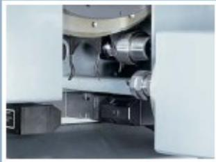
*The toolchanger is entirely enclosed. This protects the tools from both swarf and coolant. These materials can interfere with inserting tools into the spindle.*
